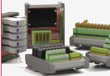
I/O conditioning accessories, including a family of Universal Termination Assemblies (UTAs) that provides signal conditioning, isolation or disconnect, single-point power distribution and more, for any field device, signal or voltage.
